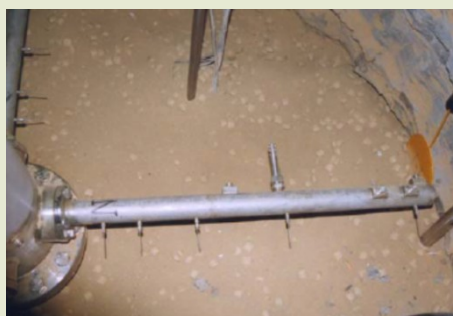
Figure 69 – RESEAL test: tube instrumented for total and pore pressure, relative humidity and temperature measurements (RESEAL II, 2009).
