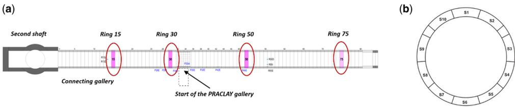
**Fig. 4.** (a) Position of the three instrumented rings in the Connecting Gallery. (b) Numbering of the segments in one ring (6-gauge segments: S2, S3, S5, S7, S9 and S10; 12-gauge segments: S1, S4, S6, S8). Source: modified from Verstricht *et al.* (2022), ©2022, with permission from Elsevier.
