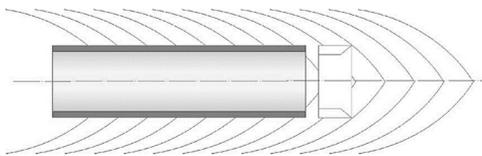
**Fig. 19.** Schematic representation of the encountered shear planes during the construction of the Connecting Gallery. Source: reprinted from Mertens *et al.* (2004), ©2004, with permission from Elsevier.
