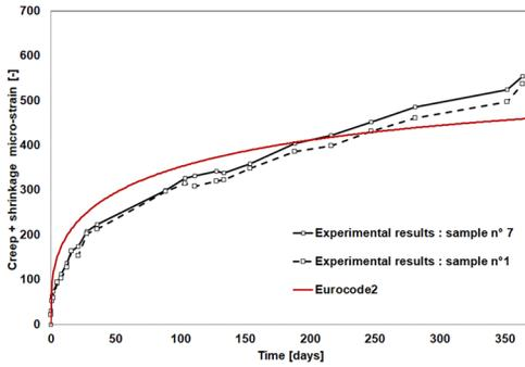
**Fig. 20.** Comparison between the Eurocode2 model (EN 1992-1-1 2004) and the experimental results (creep and shrinkage strain) obtained at UGent (De Pauw and De Schutter 2003) for two concrete samples loaded at a constant value of 36.7 MPa during one year.
