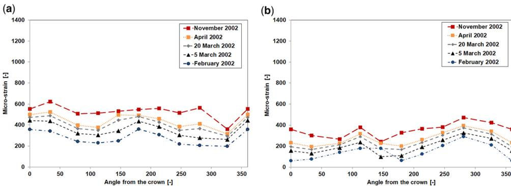
**Fig. 17.** Distribution of the strain (averaged over the segment at the intrados and the extrados) along the circumference of the tunnel in ring 30 at (a) the intrados and (b) the extrados focusing on the short-term evolution.
