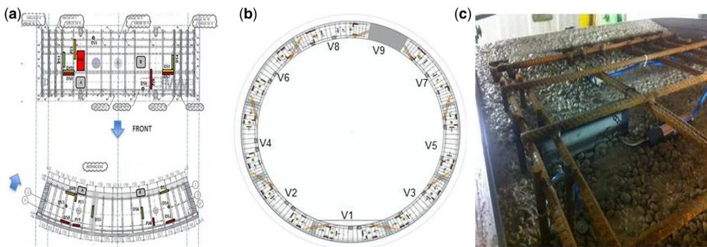
**Fig. 9.** (a) Scheme of the location of vibrating strain gauge wire and total pressure sensors in a segment and (b) in a ring (64 strain gauges and 24 total pressure sensors). (c) Photograph of the concrete pouring into the mould with the reinforcement bar and the total cells.
