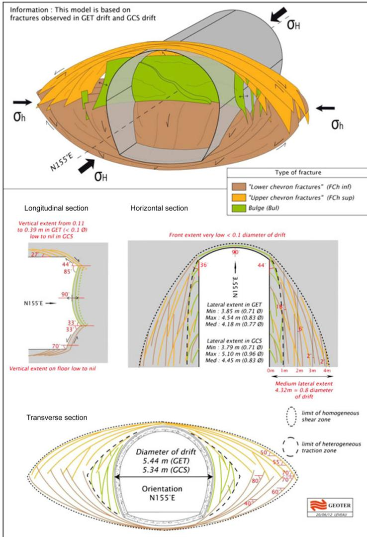
**Fig. 23.** Conceptual model for induced fractures network (shear and extensional fractures) for the gallery parallel to the major horizontal stress from Armand *et al.* (2014).
