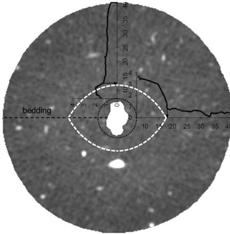
**Fig. 18.** Eye-shaped damage zone (white dashed line) around the central hole (black dotted line) of a hollow cylinder test in Boom Clay. The black curves correspond to the measured displacements, with their corresponding axis, around the central hole (Labiouse *et al.* 2014), and the black dashed line indicates the orientation of the bedding.
