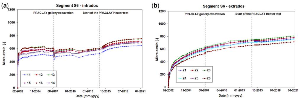
**Fig. 11.** Evolution of the strain monitored in the S6 segment of ring 30, which is a 12-gauge segment (six intrados and six extrados): (a) six strain gauges close to the intrados and (b) six strain gauges close to the extrados.
