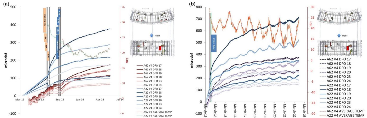
**Fig. 25.** Comparison of raw deformation (negative strain in compression) in the V4 segment lining for the two backfill grout zones: A22 (classical grout) and A62 (compressible grout zone): (a) short term during and after emplacement and (b) over 8 years.
