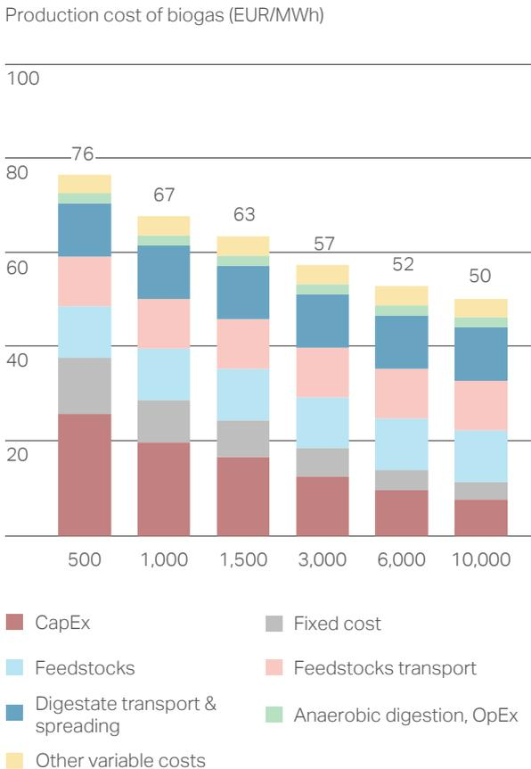
Figure 12: Cost of bio-methane production at various production capacities (as Nm<sup>3</sup>/h bio-methane). Bio-methane is compressed and prepared for grid injection. Transport costs are assumed to be proportional to the production capacity.
