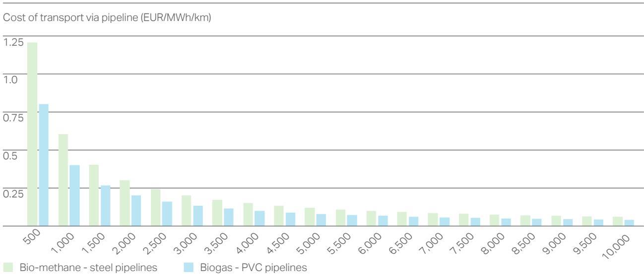
\* A maximum length of 10 km is typical for a "feeder" pipeline into a natural gas transmission or distribution system.
