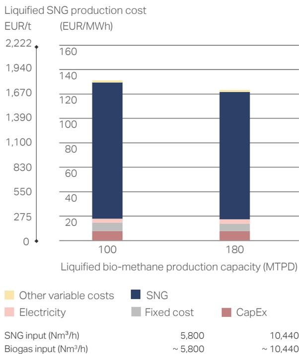
Figure 22 shows the aggregated costs for SNG liquefaction. With an electricity price of 55 EUR/MWh, we find that liquefaction of SNG is more expensive than liquefaction of biogas or bio-methane at comparable capacity. A liquefaction plant delivering 100 MTPD LBM is fed with 5,800 Nm<sup>3</sup>/h SNG. Liquefaction of this volume of catalytic SNG costs around 130 EUR/MWh or 1,700 EUR/t. In comparison, liquefaction of 100 MTPD of biogas costs only 80 EUR/MWh (1,111 EUR/t, see Figure 21).
