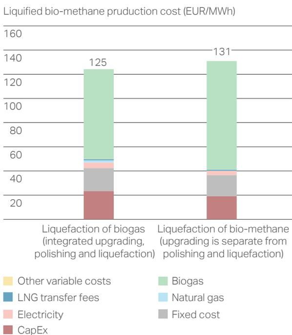
Figure 17 breaks down the cost structure of LBM production from both biogas (integrating upgrading, polishing, and liquefaction) and bio-methane (upgrading is separate from polishing and liquefaction) (Routes 1 and 2 in Section 2.1).
