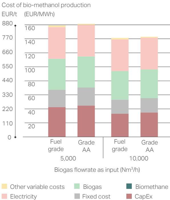
The manufacturing cost of grade 'AA' bio-methanol for a biogas capacity of 10,000 Nm³/h is 143 EUR/MWh, which is more expensive than both liquified catalytic SNG (123 EUR/MWh, see Figure 22) and liquified biogas (80 EUR/MWh, see Figure 21) at the same biogas input capacity. The manufacturing cost per tonne of grade 'AA' bio-methanol is lower than that of bio-methane due to methanol's lower energy density.
