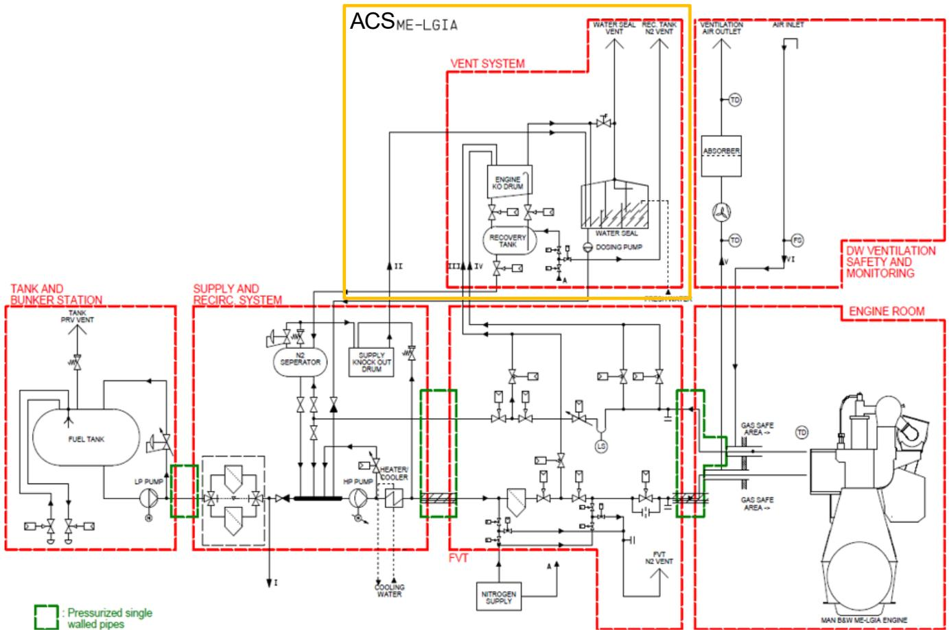
The FVT is the interface between the engine and the FSS auxiliary systems. The FVT ensures safe isolation of the engine during shutdown and maintenance and provides a nitrogen purging functionality to neutralize the system after shutdown.
