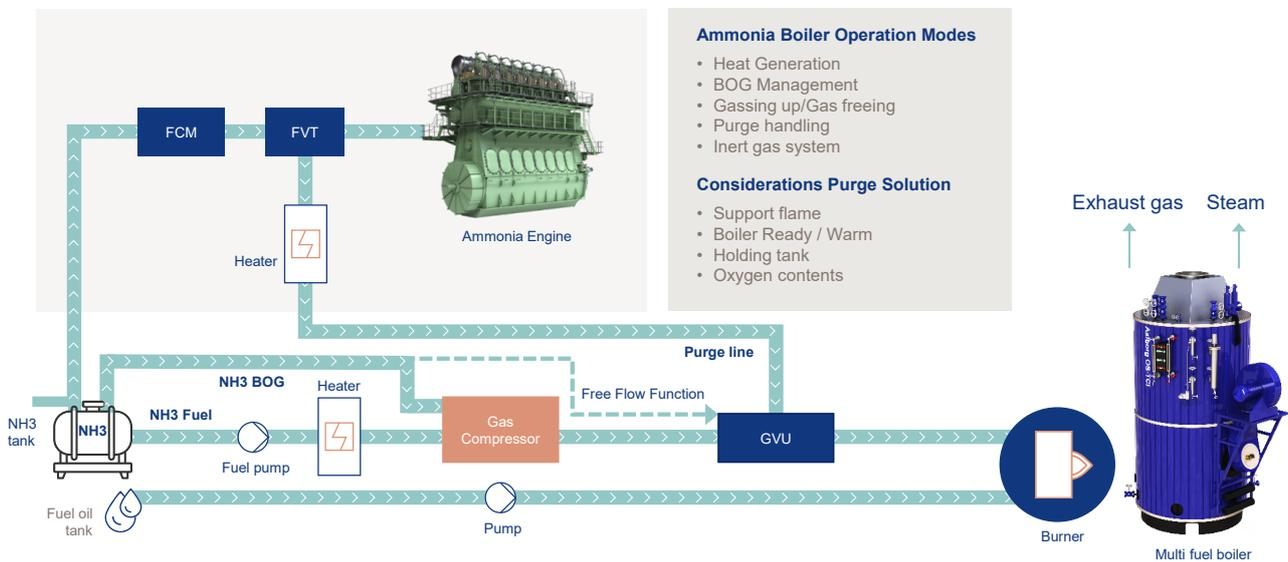
FCM = Fuel conditioning module, FVT = Fuel valve train, GVU = Gas valve unit.
