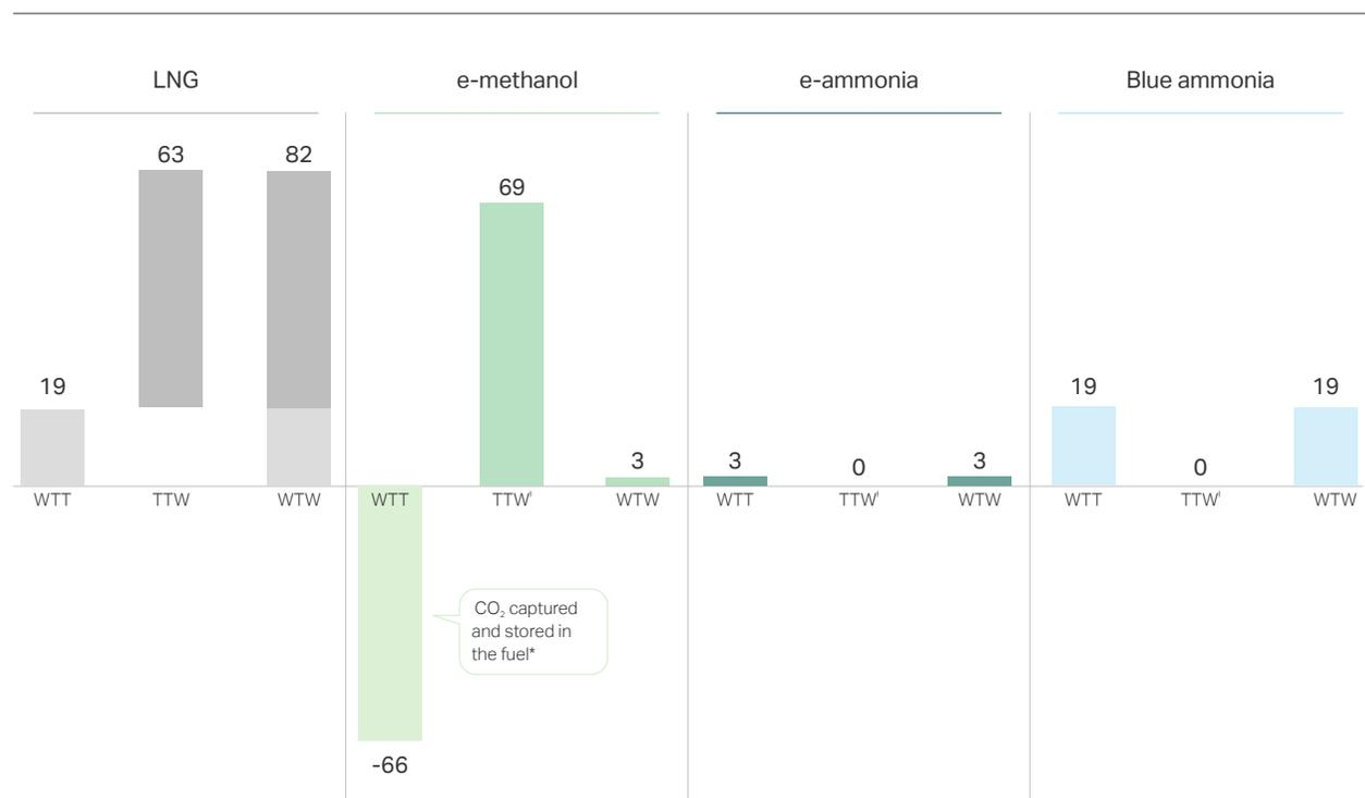
Well-to-wake (WTW), well-to-tank (WTT), and tank-to-wake (TTW) emissions from LNG, e-methanol, e-ammonia, and blue ammonia. WTT, TTW, and WTW values are in kgCO<sub>2</sub>.eq/GJ.
