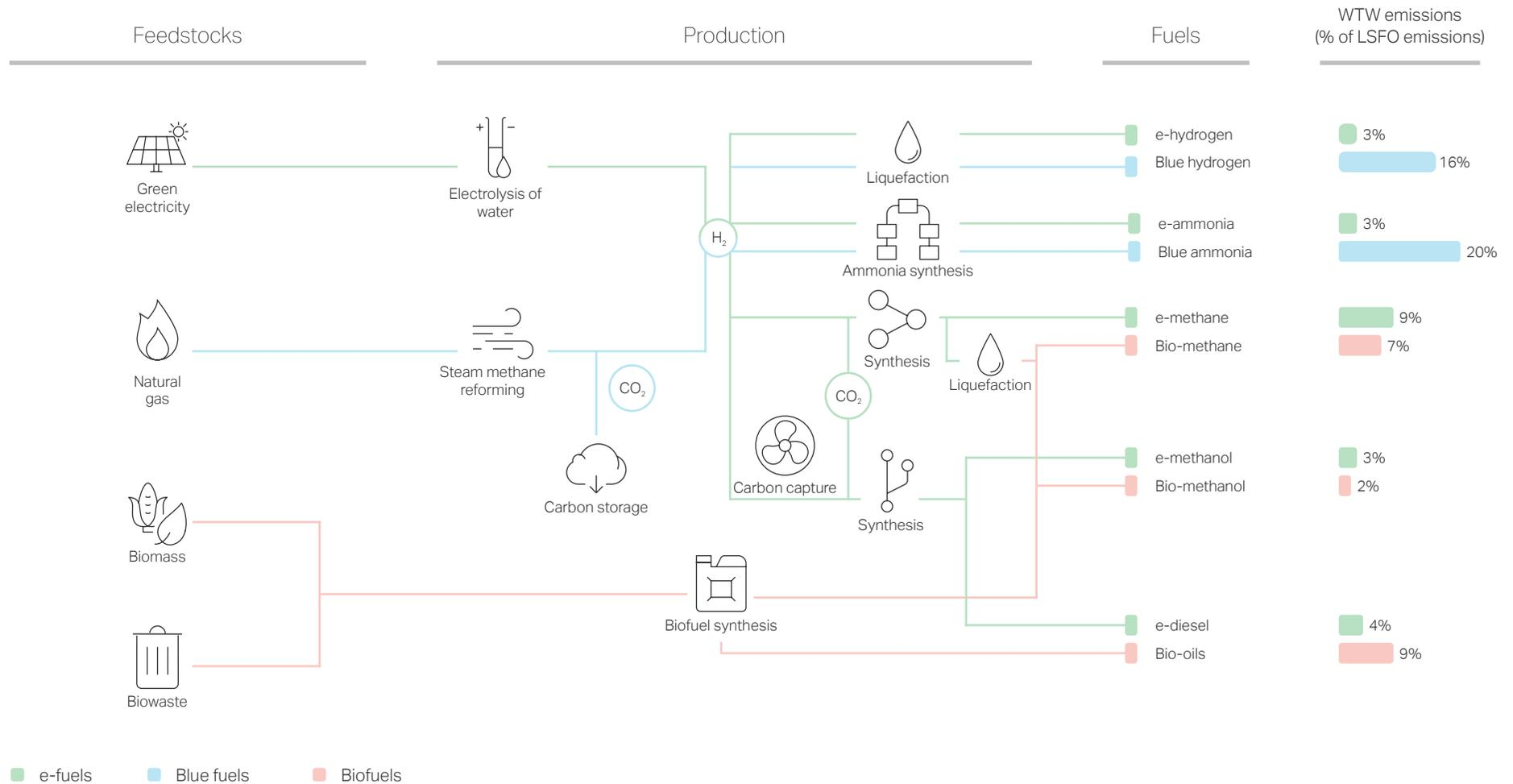
Note: Only key processes are included; Methane slip in upstream production processes of blue ammonia and bio-methane are factored into emissions estimations based on the technology maturity levels forecasted for 2030. Emissions are well-to-wake emissions as a percentage of LSFO emissions of 93gCO<sub>2</sub>,eq/MJ in 2030. Data source: NavigaTE, MMMCZCS.
