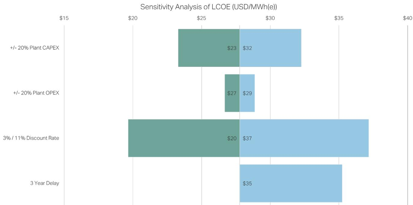
**Figure 6** Sensitivity analysis of the effect of techno-economic inputs on the Levelized Cost of Electricity.
