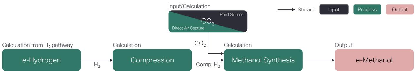
Production pathways for various fuels are set-up as a series of connected processes, see Figure 9 below.
