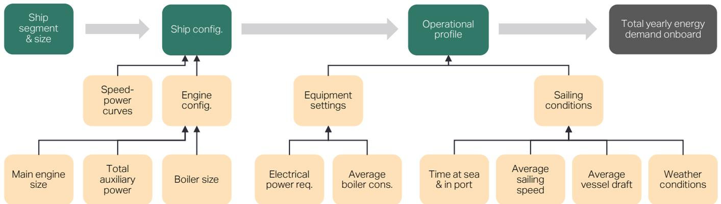
impact of replacing individual elements of a vessel with more energy efficient technology. As an example, the implementation allows for estimating the impact of changing from an auxiliary internal combustion engine to a fuel cell and what impact that has on the cost and emissions.
