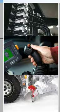
The hydraulics and related control system developed by Sisu were thoroughly tested and belong to the most versatile ones on the market. In the design of hydraulics, attention is paid to new accessories and their requirements, for which information transfer based on the bus technology enables simple operation with a display screen to guide the driver. As a result, the driver can focus on controlling the vehicle instead of the accessory functions.
