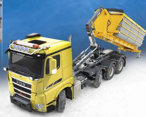
Thanks to the frame structure and axle system, the SISU Roll is stable and agile to drive. The liftable axles, combined with good turning ability, make the vehicle excellent to drive.
