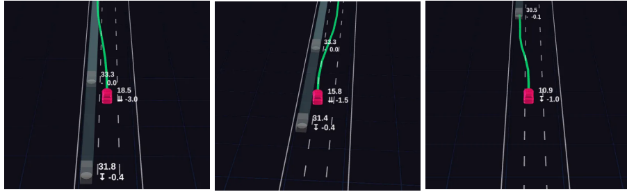
Fig. 7: Here we see a failure case of our model. The agent makes a bad decision to initiate a lane change before making a last minute adjustment to avoid collision. While collision is avoided, this is still unsafe behavior.
