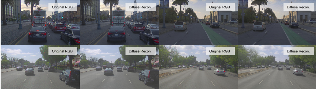
Figure A18: View-independent reconstruction results for LightSim. Shadows are baked at this stage, which are then mitigated by neural deferred rendering. The relighting failure cases for the last example are shown in Fig. A17.
