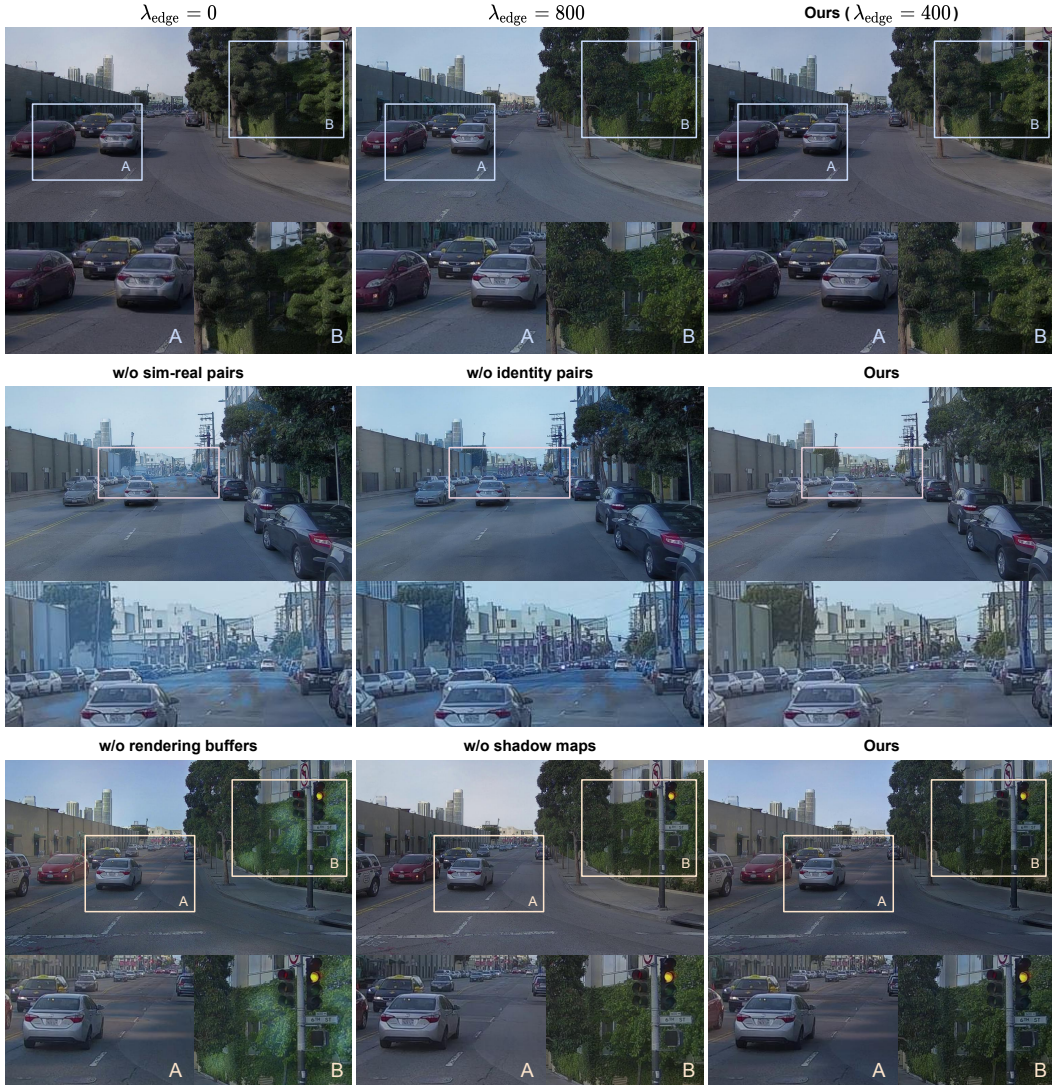
Figure A10: Additional ablation study on neural deferred rendering. LightSim can simulate intricate lighting effects (highlights, shadows) while maintaining realism.
