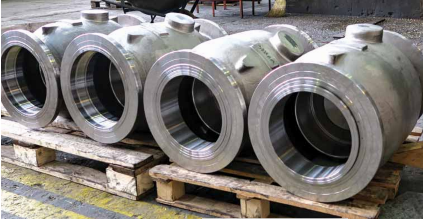
Stainless Steel needle valves bodies DN 200 After partial machining in our workshop
