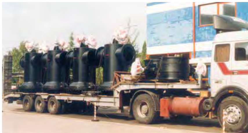
▼ Double flanged sleeve valves DN 800 PN 25
