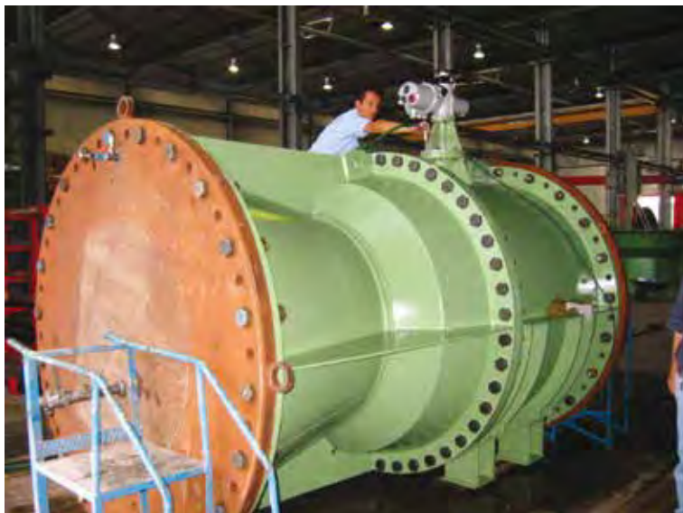
Needle Valve DN 1400 PN 10 Body pressure test
