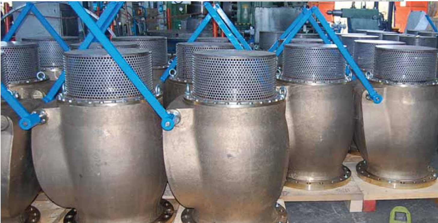
Vacuum breakers (Al-Br) DN 300 ASME/ANSI 150 Saudi Arabia
