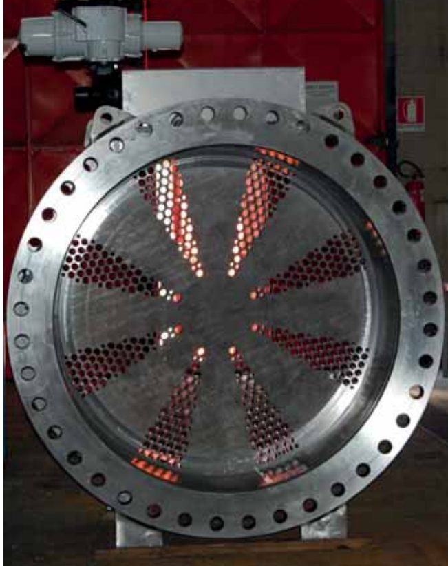
Multijet rotative valve DN 1500 PN 25 Saudi Arabia
