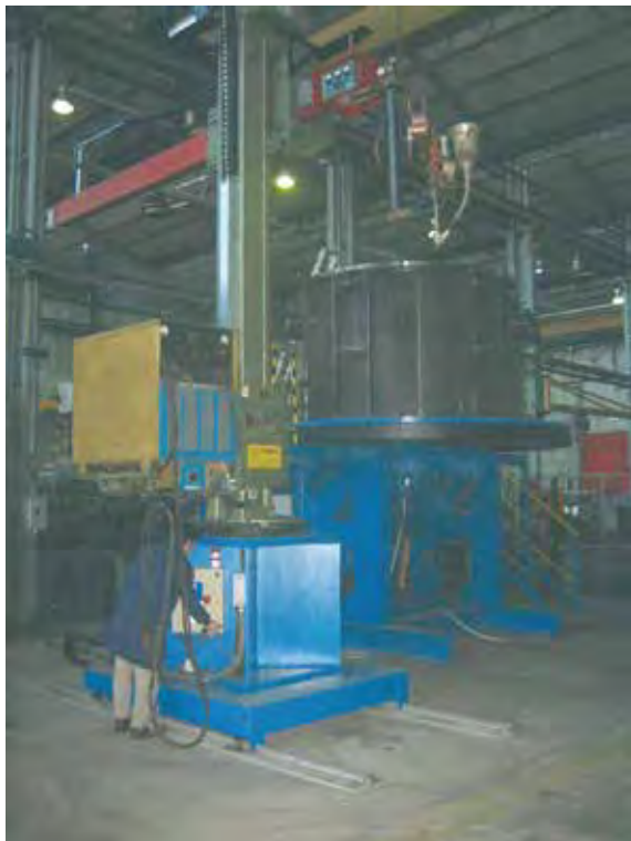
Submerged arc welding process for Butterfly valve body
