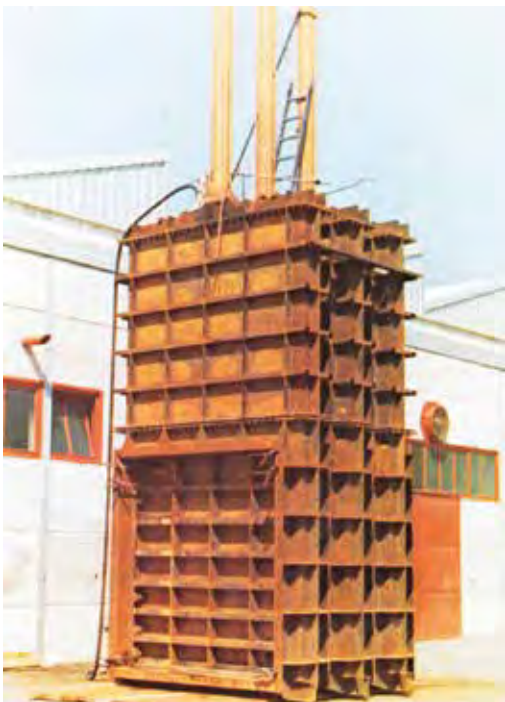
High Pressure Outlet Slide Gates 2550x2500 mm. Head 30 m.w.c. Welded carbon steel
