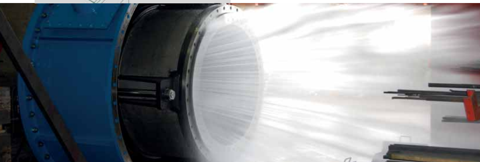
Fixed cone valve DN 1550 PN 16 Under Final Acceptance Test (FAT) in our workshop
