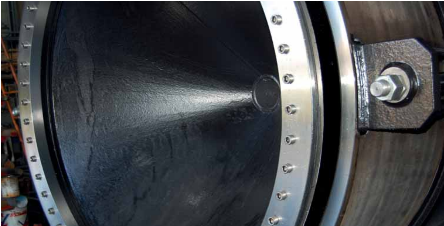
Fixed cone valve DN 1000 PN 10 Under assembling in our workshop
