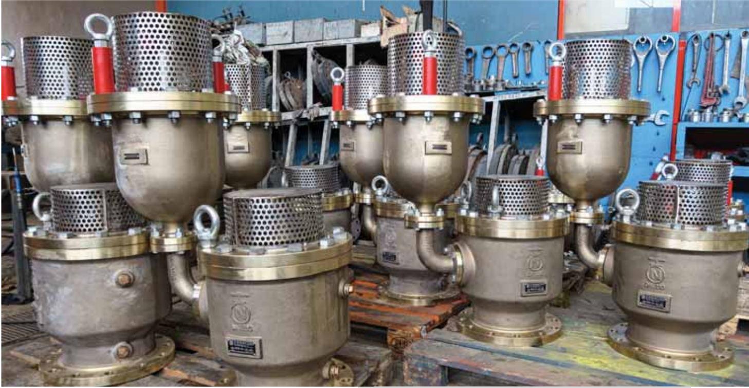
Combination air valves (Al-Br) DN 200 ASME/ANSI 150 Saudi Arabia
