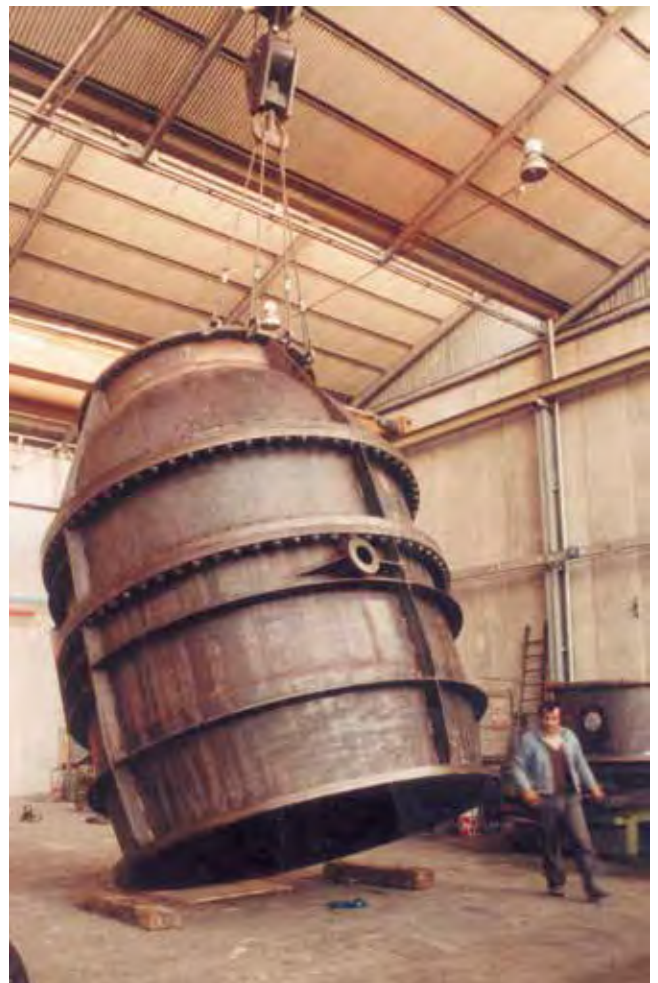
Needle valve body after welding process DN 3000 PN 10
