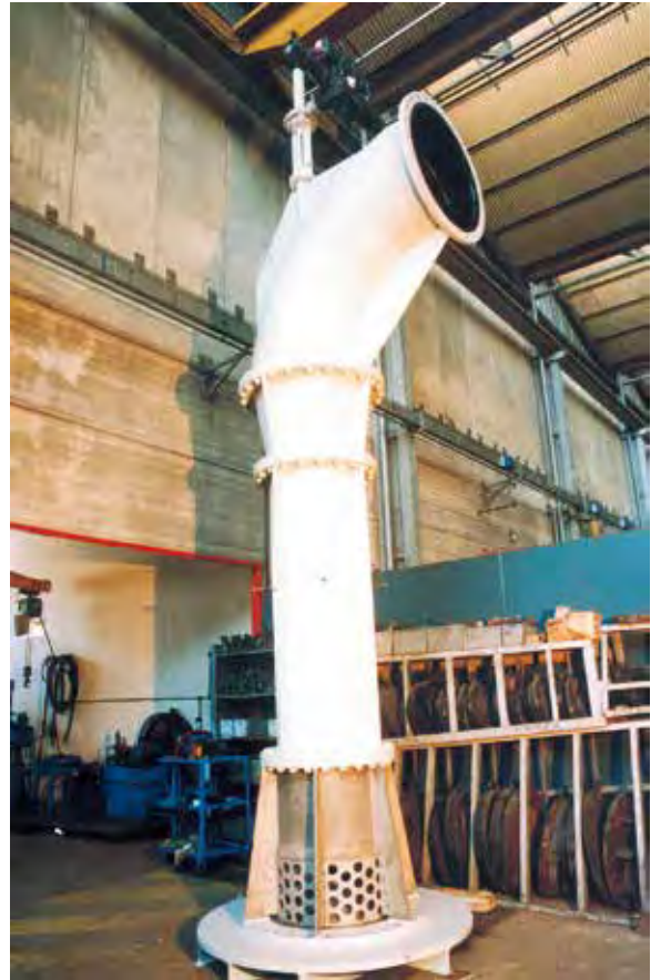
▼ Submerged discharge valve, Vertical Sleeve type DN 600 PN 25 Welded carbon steel
