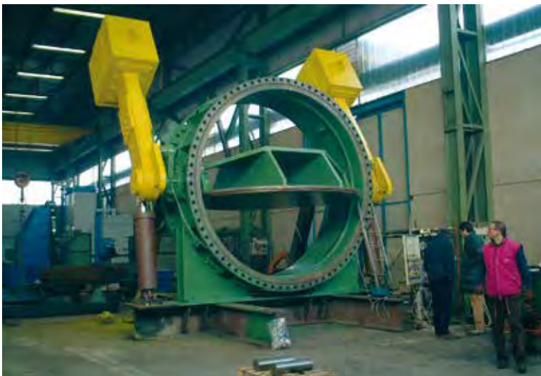
▼ Counterweight Butterfly Valve DN 2000 PN 16 for Hydropower by-pass
