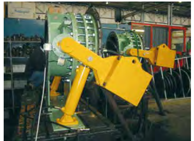
Counterweight Butterfly Valve DN 2000 ANSI 400 for Hydropower by-pass
