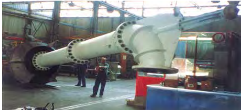
► High Pressure Control Valve DN 400 PN 25 Welded carbon steel
