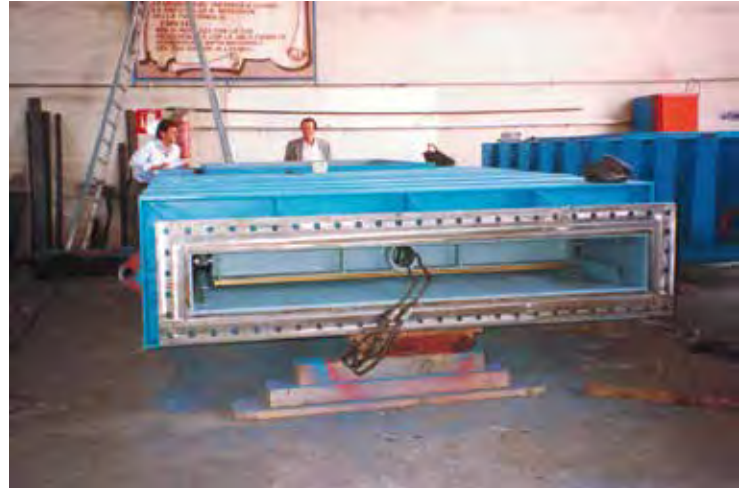
High Pressure Outlet Slide Gate 3000x3000 mm Head 45 m.w.c. Welded carbon steel
