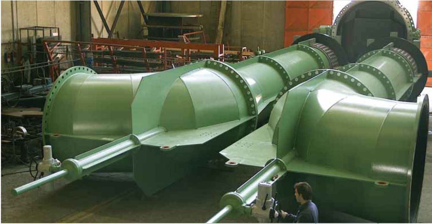
Submerged vertical sleeve valves DN 2000 PN 16 Under Final Acceptance test (FAT) in our workshop
