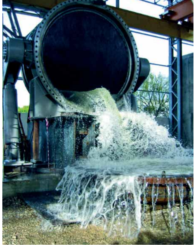
Butterfly valve DN 3550 PN 6 Morocco
