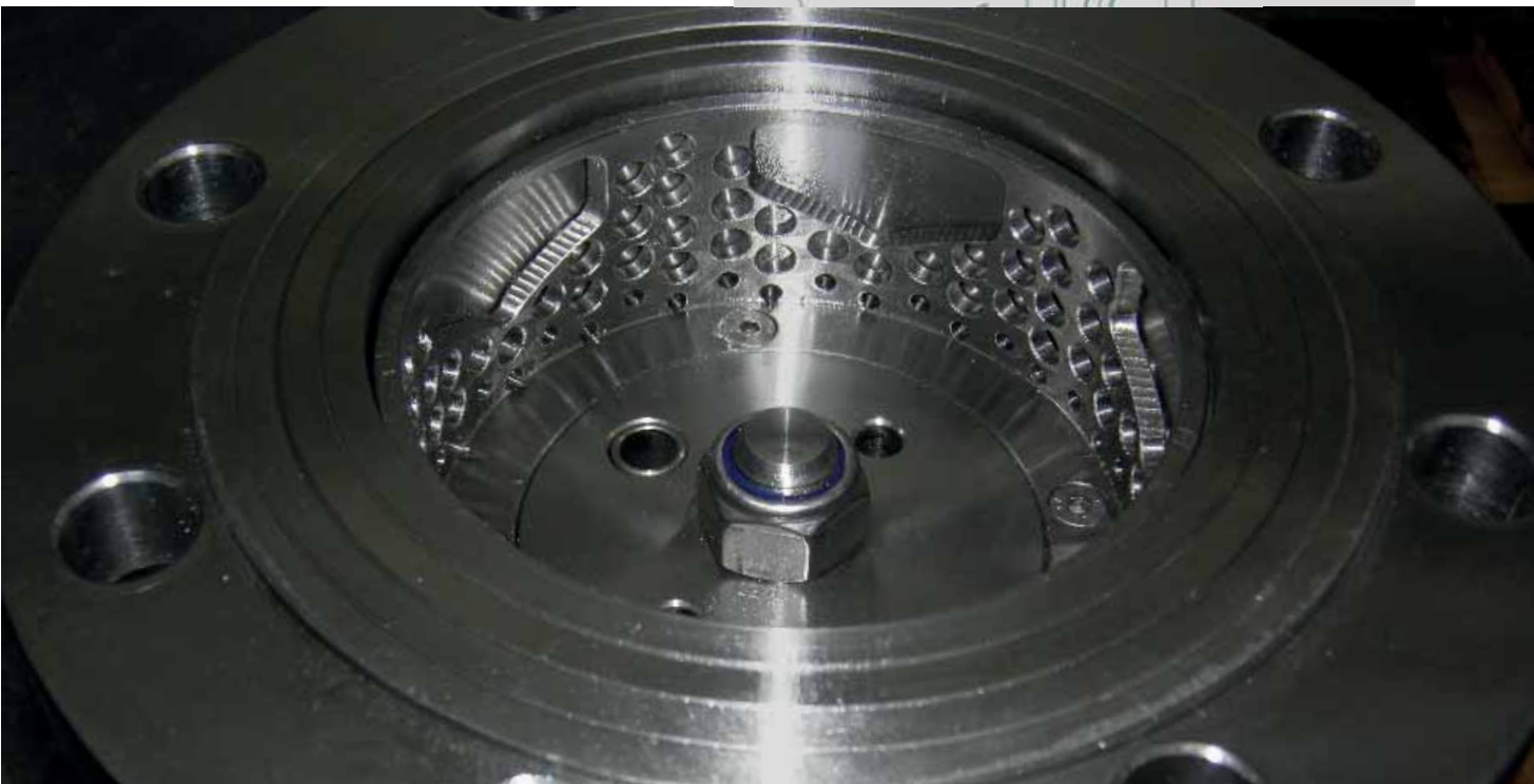
Needle valve: detail of special anti-cavitation trim
