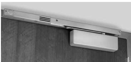
The Power Track® Series combines the function of a single-point electromechanical door holder with the proven reliability of a 7500 Series door closer. The track assembly contains an arm slide and solenoid operated hold open mechanism and is available with or without an integral smoke detector.
