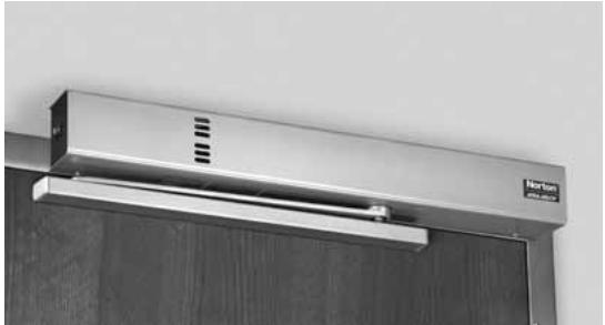
The 7200 Series is a multi-point electromechanical closer/holder that provides flexibility to installers and facility managers. Shipped standard with selective hold open, the 7200 Series is designed to hold the door open at any point up to 180°. Available for push or pull side mounting, these units can be ordered with integral smoke detectors or remote wireless door releases.
