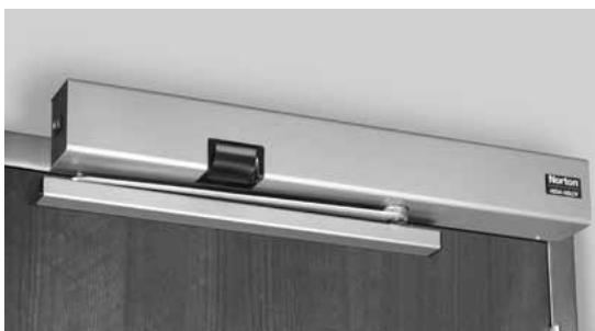
The 7100SZ Series SafeZone door closer safeguards occupants throughout a variety of facilities with the detection of movement through doorways and intelligent door control functions. A multi-point electromechanical closer with a programmable motion sensor allows the door to open manually and remain open when one or more people travel through the opening.
