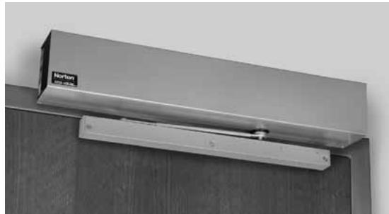
The 5700 Series design is based on ease and simplicity. This unit installs in minutes rather than hours and consists of three basic components: inverter, motor and Norton's 1601 closer body. Quiet and dependable, the 5700 meets the requirements of the Americans with Disabilities Act (A.D.A.) and ANSI/BHMA A156.4. Available push or pull side mounting, this unit is perfect for applications that don't require special features but demands reliability.
