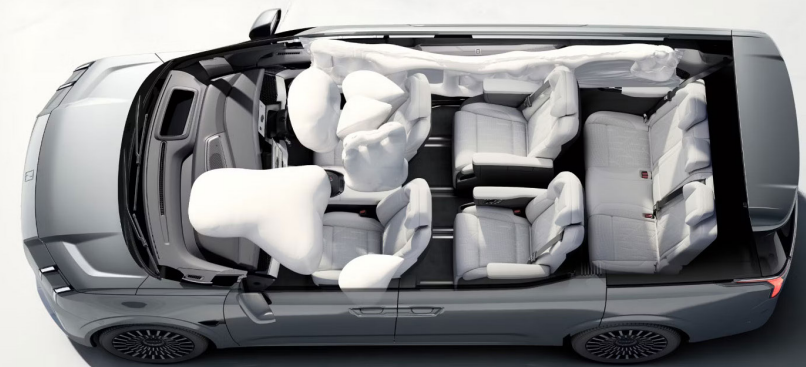
7-airbag system covers all three rows
