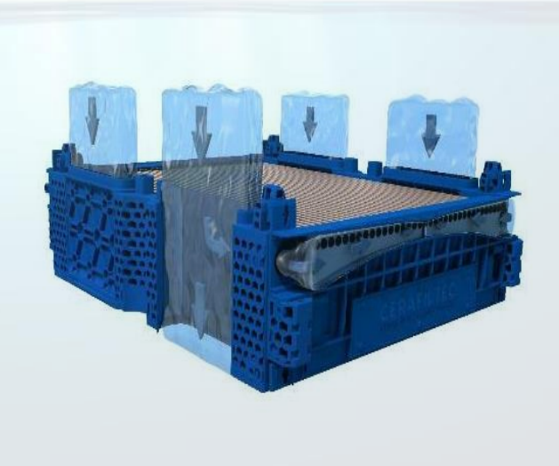
Figure 16: Module principle of the filtration and backwash processes.
