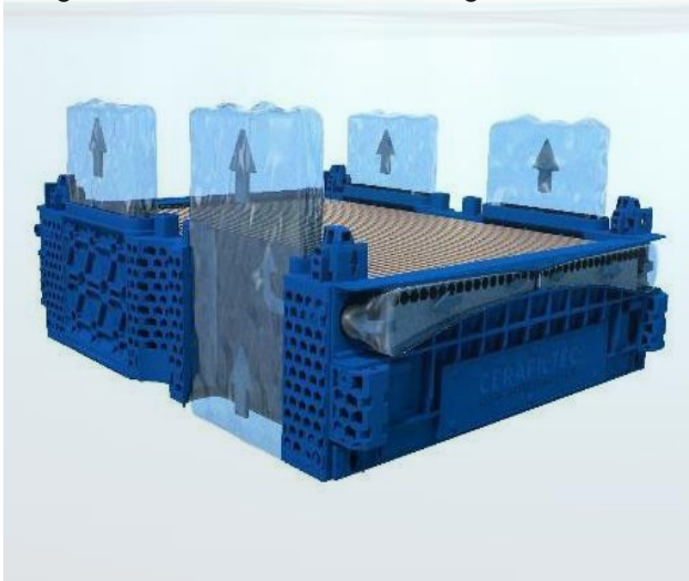
Figure 16: Module principle of the filtration and backwash processes.
