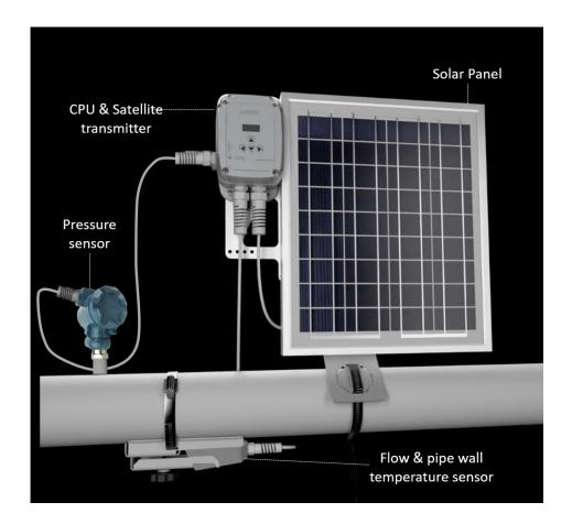
The primary mechanism for reading activity in the pipe is through the ultrasonic acoustic waves sent and received by the transducer. These waves are powerfully transmitted through the pipe wall, any scaling or paraffin buildup and reflect off of the many bubbles or solids present in the flowstream.
