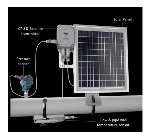
The primary mechanism for reading activity in the pipe is through the ultrasonic acoustic waves sent and received by the transducer. These waves are powerfully transmitted through the pipe wall, including any scaling or paraffin buildup and reflect off of the many bubbles or solids present in the flowstream.
