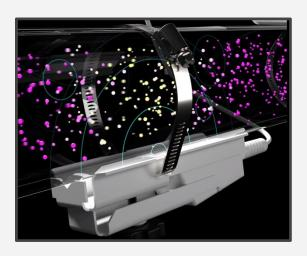
The proprietary onboard processor performs a spectral frequency analysis of the waves to calculate a flow profile. From the profile of these sound waves, a mix of on-board and cloud-based algorithms compute a fluid velocity in the pipe.
