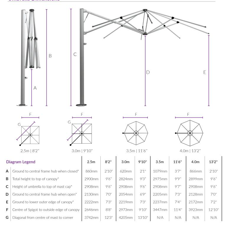
\*Free-Standing Base installations will add 165mm | 6" to the height and surface plates will add 12mm | ½" to the height. Adding Free-Standing Base wheels also will add a further 45-80mm | 2-3". All sizings are +/- 2.5mm | 3/42" and subject to change without notice.
