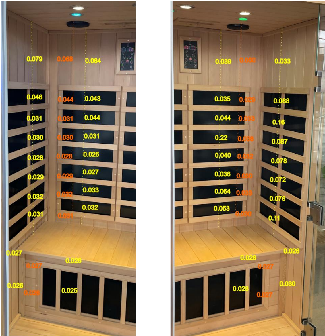
Fig 2. Magnetic field measurements in the Linear 2-person sauna. Left side of the sauna shown on the left, right side of the sauna on the right. Figures show the magnetic flux density in microtesla ( \mu\text{T} ). Figures in yellow show the values next to the heater panels at the rear and sides of the sauna, figures in orange show the field at the approximate position of the centre of the body of someone sitting in the sauna.
