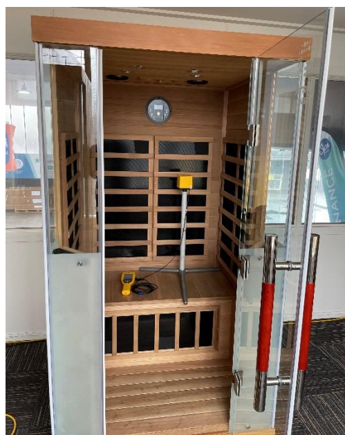
Fig 4. Position of the measurement probe on the right side of the Prestige sauna for recording the magnetic field against time.
