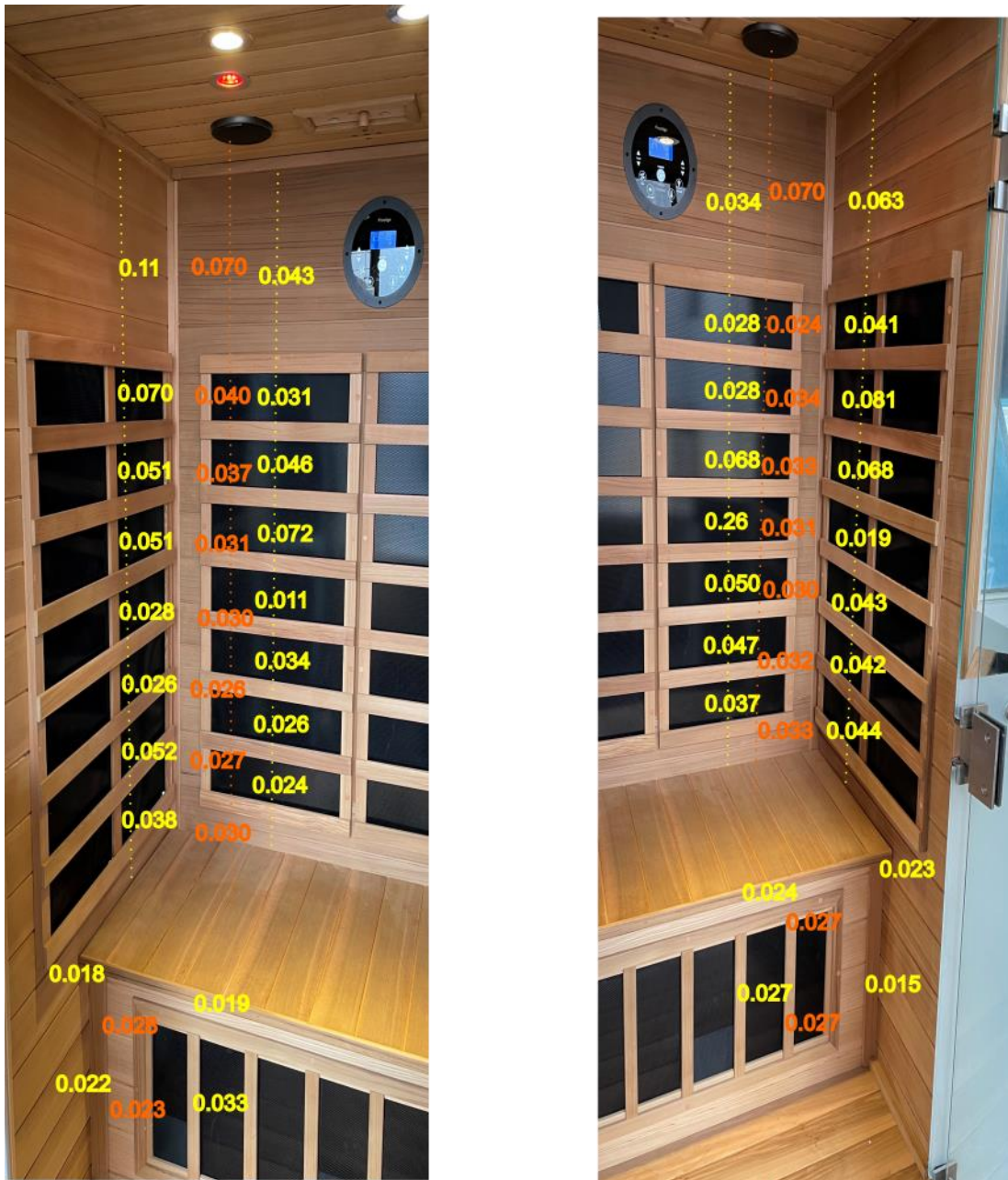
Fig 1. Magnetic field measurements in the Prestige 2-person sauna. Left side of the sauna shown on the left, right side of the sauna on the right. Figures show the magnetic flux density in microtesla ( \mu\text{T} ). Figures in yellow show the values next to the heater panels at the rear and sides of the sauna, figures in orange show the field at the approximate position of the centre of the body of someone sitting in the sauna.
