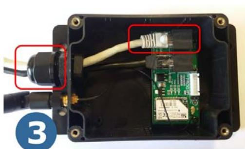
**3** Feed existing cable through gland & connect into spare socket labelled RJ1, tighten gland and screw lid back in place
