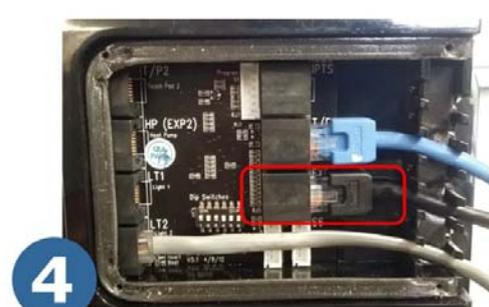
**4** Connect black data cable from SpaLINK module into EXP1 socket
