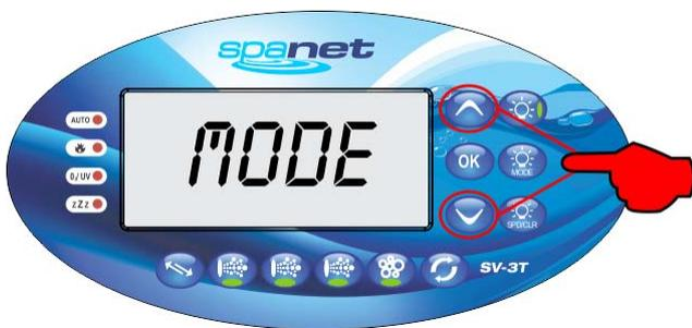
**Step 2:** Press the DOWN button multiple times until display shows [WIFI]
