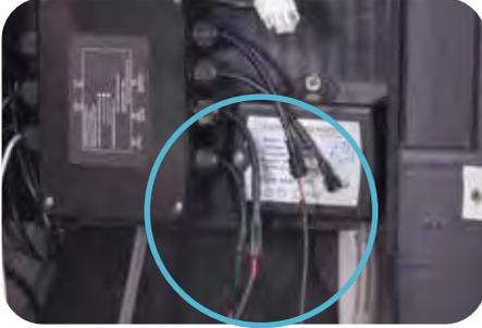
**Step 7: Connect power supply to amplifier.**
