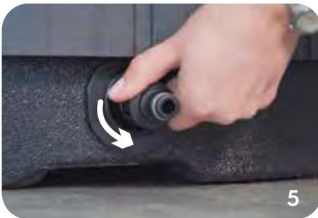
Replace the cap with the hose nozzle and twist until it is hand tight
