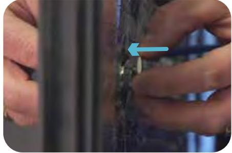
Complete the final connection by plugging the button into the connector on the back.
