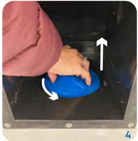
Remove the filter counter-clockwise
