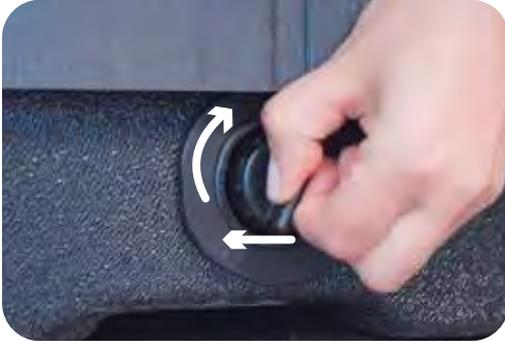
If it is open, twist and press in the drain cap.
