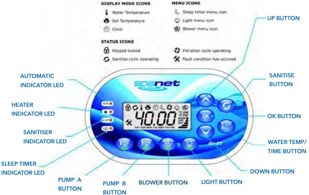
**AUTOMATIC INDICATOR LED:** This LED will turn on whenever the filtration pump is in automatic mode.
