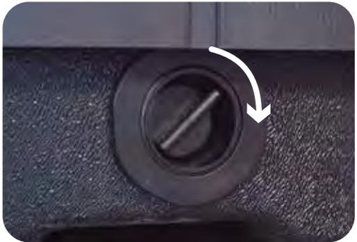
Tighten the cap. Close drain valve.
