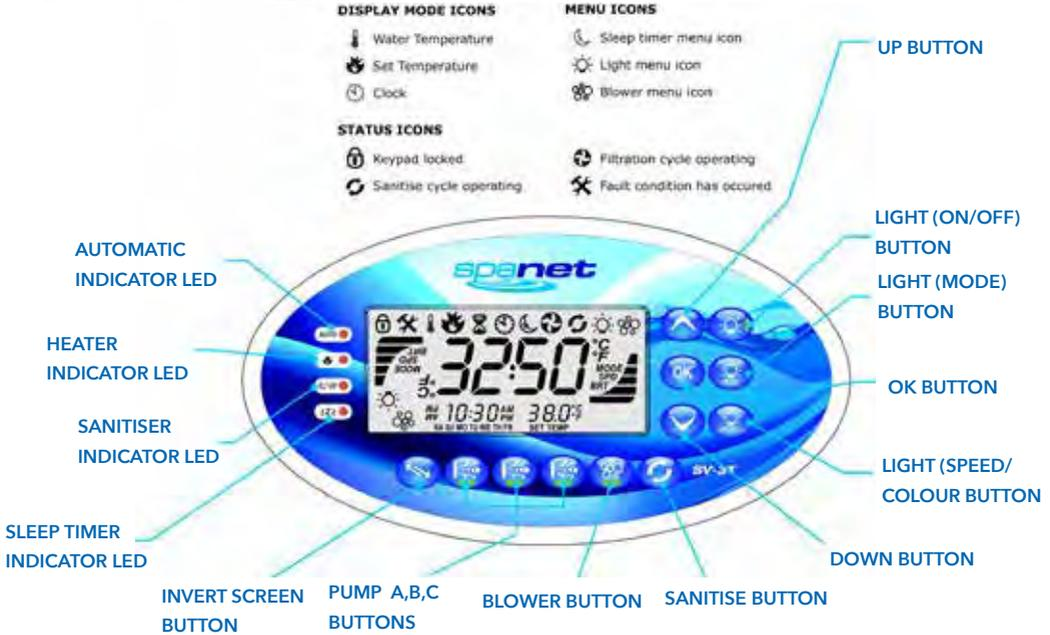
**AUTOMATIC INDICATOR LED:** This LED will turn on whenever the filtration pump is in automatic mode.
