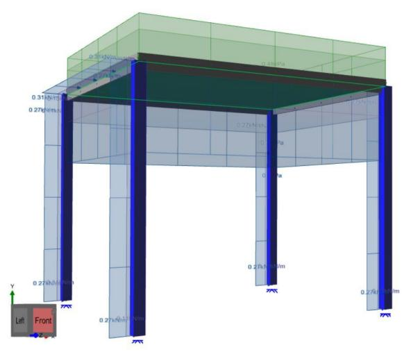
Figure 1 - Load cases applied to the Structure
