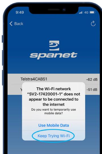
**Note:** *If no WiFi network found, relocate SmartLink™ module to a better position and use the refresh button to conduct a new WiFi scan to see if signal has improved. Signal strengths closer to 0 are stronger.*
