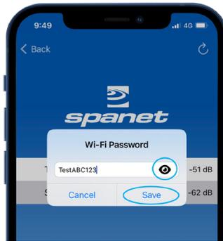
**Note:** Take care when entering password, the SmartLink™ module or app cannot check or verify the password. It relies on correct entry. If the password is incorrect, you must delete the spa instance and start the setup process again.
