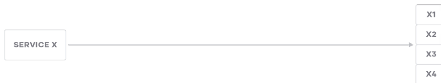
Figure 27: Service endpoint resolution without Layer 7 Traffic Management.
