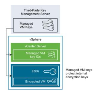
During the encryption process, different vSphere components interact as follows.
