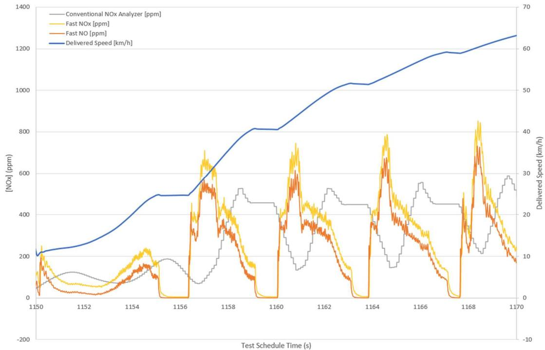
**Figure 3: Detail of transient NO<sub>x</sub> during hard accelerations and gear changes compared with a conventional NO<sub>x</sub> analyzer**
