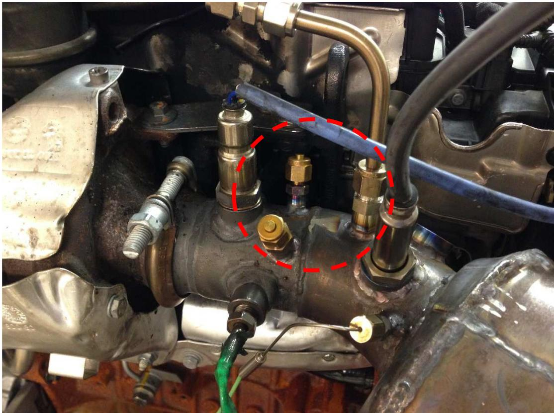
**Figure 1: Engine-out sampling points for fast NO and NO<sub>x</sub>**
