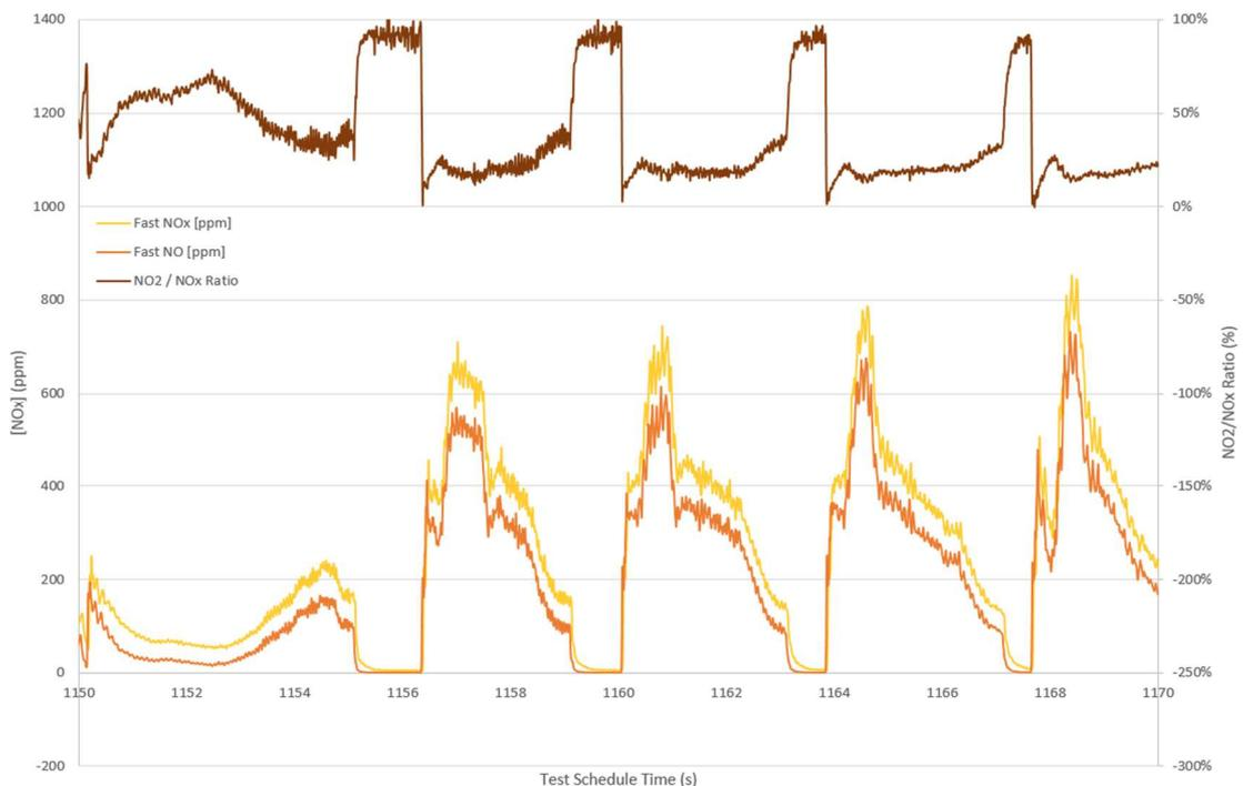
**Figure 4: Transient NO<sub>x</sub> during hard accelerations and gear changes**
