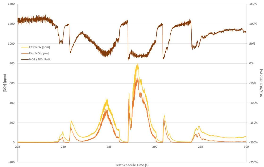
**Figure 6: NO<sub>2</sub>: NO<sub>x</sub> ratio during moderate transients**
