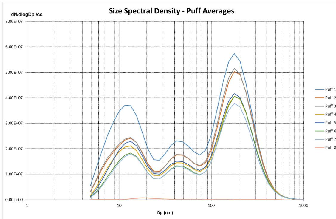
There is greater variability observed in this test, compared with the automatically triggered e-cigarette previously tested in application note 12. The short interval between puffs means that the device will not have cooled to equilibrium conditions between puffs, and indeed there is a systematic trend observed in the mass concentration.
