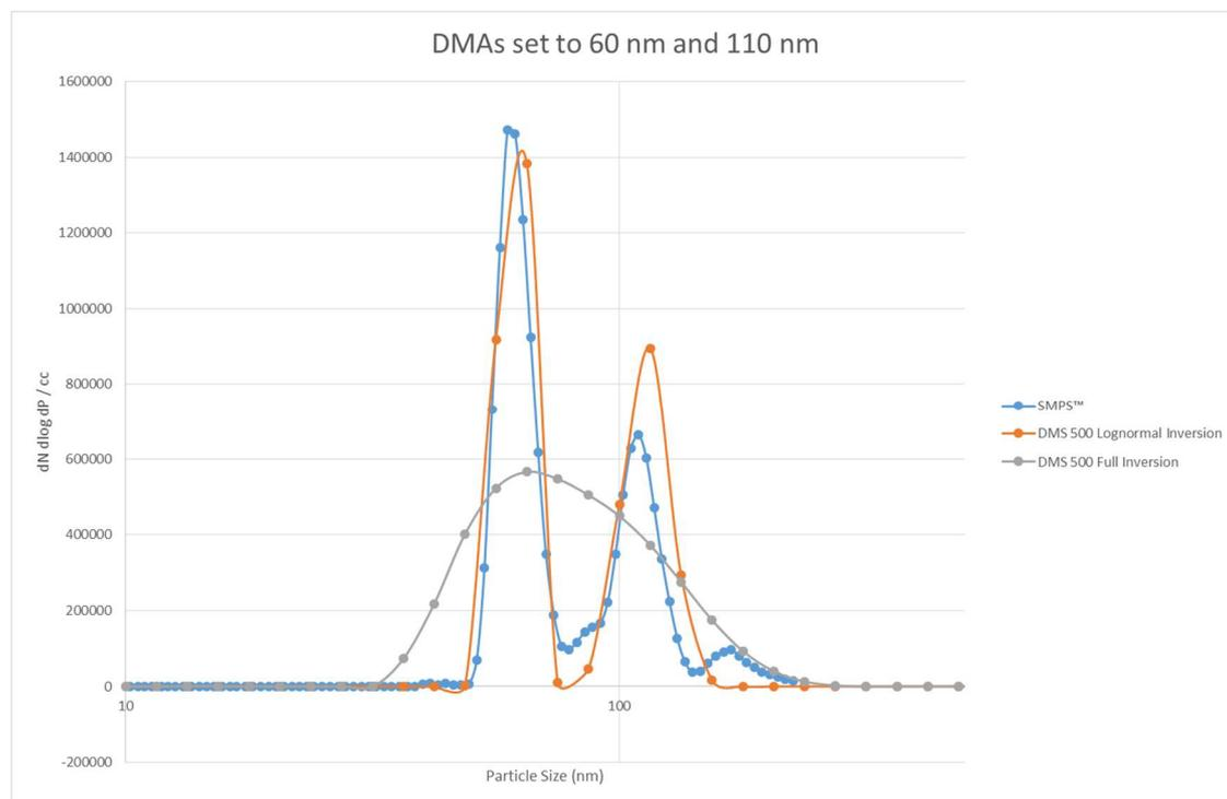
In each case, both the full spectral and bimodal lognormal inversions of the DMS500 are shown. The lognormal inversion is capable of much higher resolution than the full inversion, and the DMA modes are resolved to be almost as narrow as the SMPS can. The full unconstrained inversion does indeed show less resolution than the SMPS, but is still capable of resolving multiple peaks per decade of size range.
