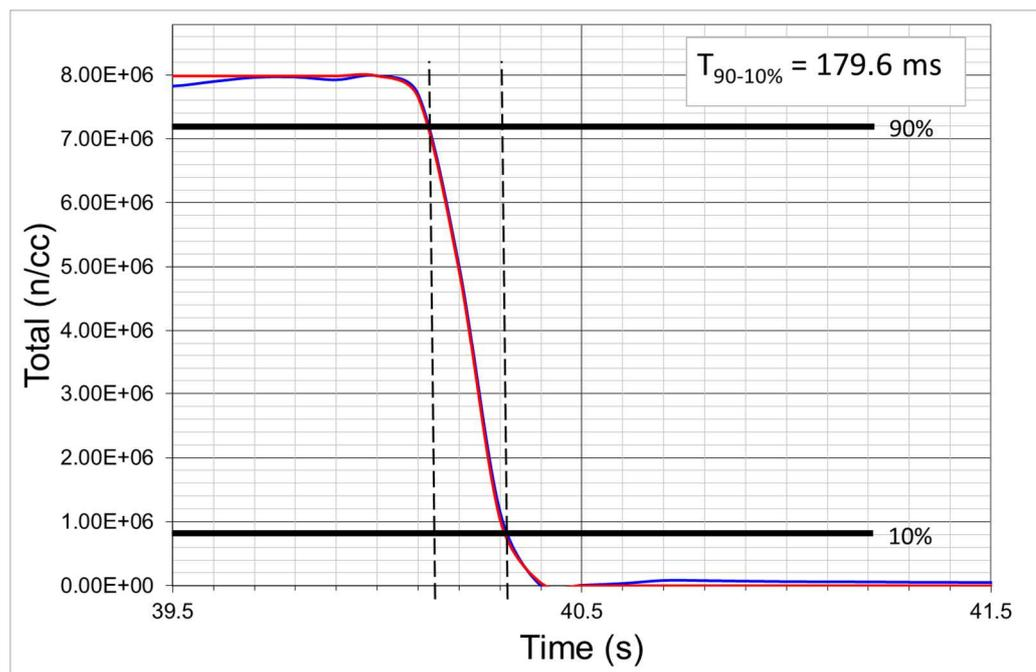
Curve fitting of this data shows that the  $T_{90-10\%}$  response time is 180 ms. Coupled with a data rate of 10Hz (appropriate for the physical response of the detectors) this demonstrates the DMS500's ability to resolve highly transient features.
