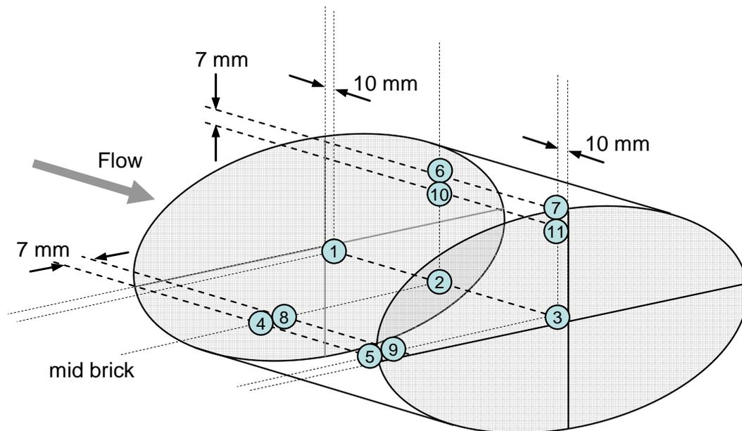
The maximum temperatures generally occur near to the axis at the rear of the brick and the highest temperature gradients typically also occur near the rear of the brick close to the edge (adjacent to the can).
