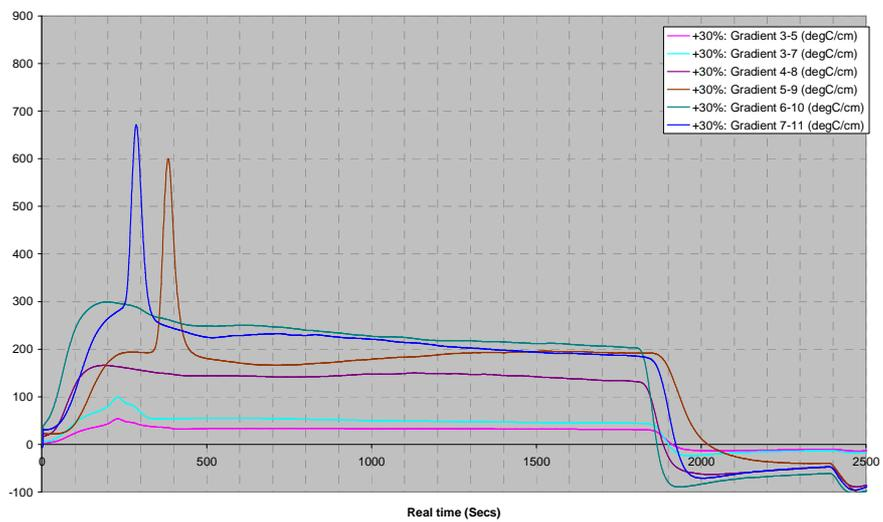
It will be noted that the radial temperature gradients are significantly higher than the axial temperature gradients (in terms of °C/cm)
