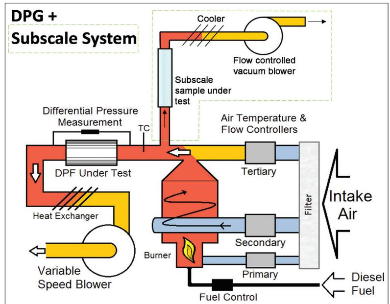
The full range of tests: loading, filtration, regeneration and flow testing can be run on the subscale parts.
