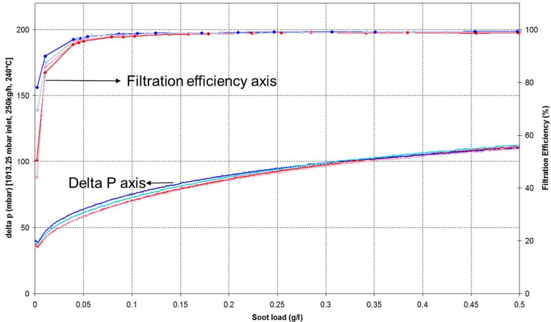
Figure 1: The back pressure and filtration efficiency results from two coated GPFs showing repeats as light colours.
