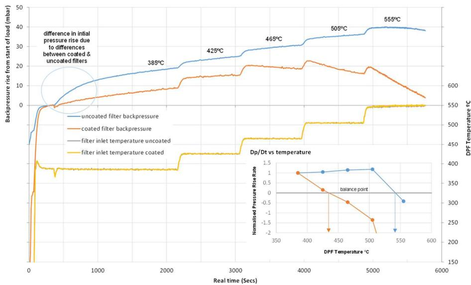
Figure 4 - balance point testing results
