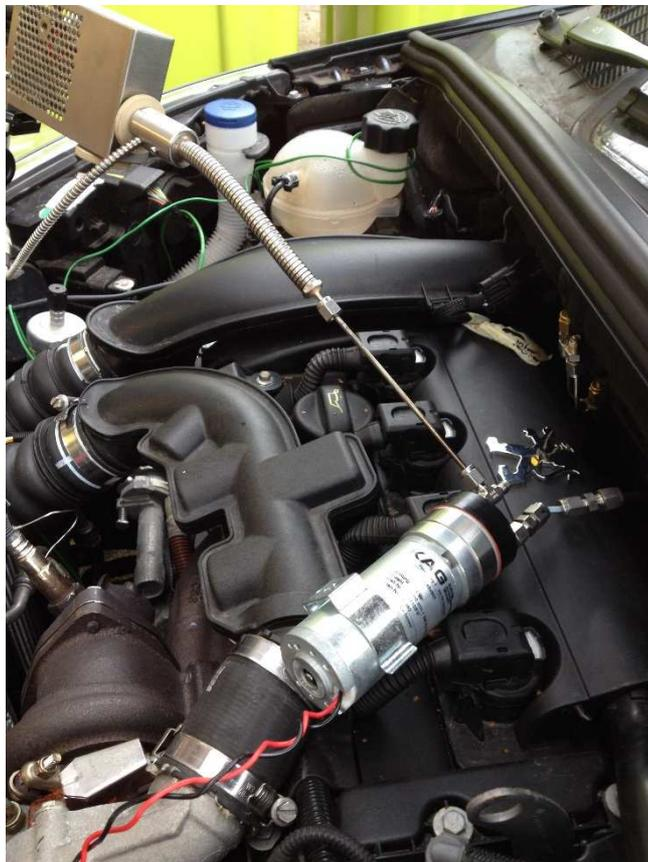
A solution is to use a small volume pump to extract just enough sample gas from the intake manifold to satisfy the flow requirements of the fast FID and then use the fast FID to sample from the pump’s exhaust. By sourcing a pump which runs hot enough to avoid any significant liquid HC hang-up, but with small enough trapped volume to avoid slowing down the resulting response time too much, a system has been designed which yields a T10-90% response time of less than 100 milliseconds.
