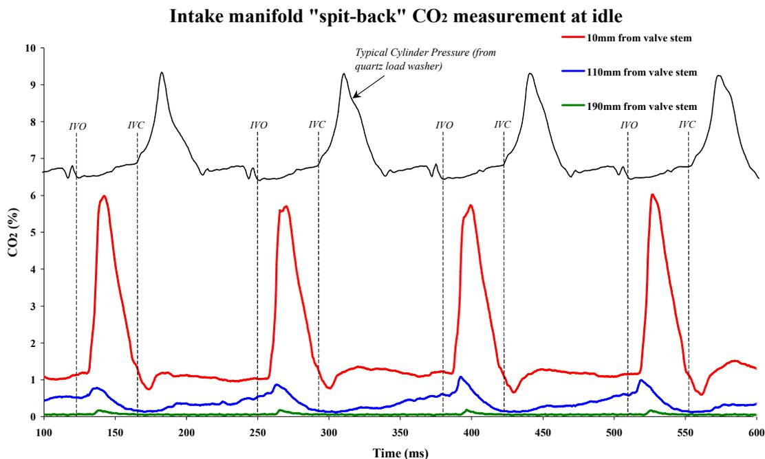
Figure 2: CO<sub>2</sub> penetration into the intake
