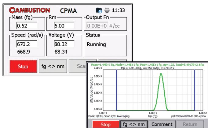
Users may set a single mass setpoint (voltage / rotation speed are then calculated automatically) or set up an automatic mass scan between specified extremes.
