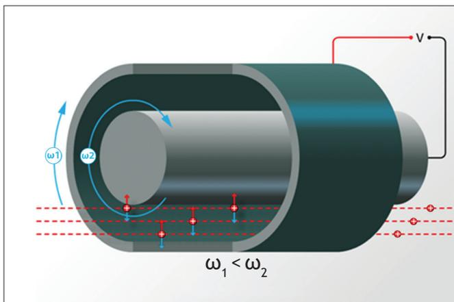
This offers improved transmission efficiency even at high resolution. A constant force balance across the classification zone ensures particles are evenly classified, even if they do not enter exactly in the centre of that zone.
