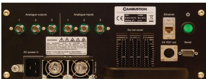
The CPMA has an RS232 port and three analog input channels for easy experimental setup. The CPMA can connect to many standard detectors such as CPCs using in-built communications settings, or the user can program custom settings. This allows the set up of experiments and results plotting in real time. The CPMA serial interface is currently out-of-the-box compatible with: Airmodus A20 CPCs,
