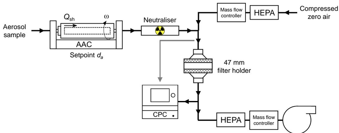
Figure 2: Schematic for measuring size-resolved particle penetration
