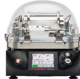
It may be considered an equivalent instrument for particle mass to the Differential Mobility Analyzer (DMA), which allows selection of particles according to their electrical mobility (drag:charge ratio).
