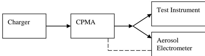
Note that it is the output function (in mg/m<sup>3</sup>) which is the key comparator; the mass setpoint, assuming a single charge ( $M_{+1}$ , in fg) of the CPMA is not directly relevant. This is because the instrument under test will measure *all* the  $M/n_q$  states from the CPMA, and thus it is not true that the selected calibration aerosol is monodisperse at the setpoint mass  $M_{+1}$ .
