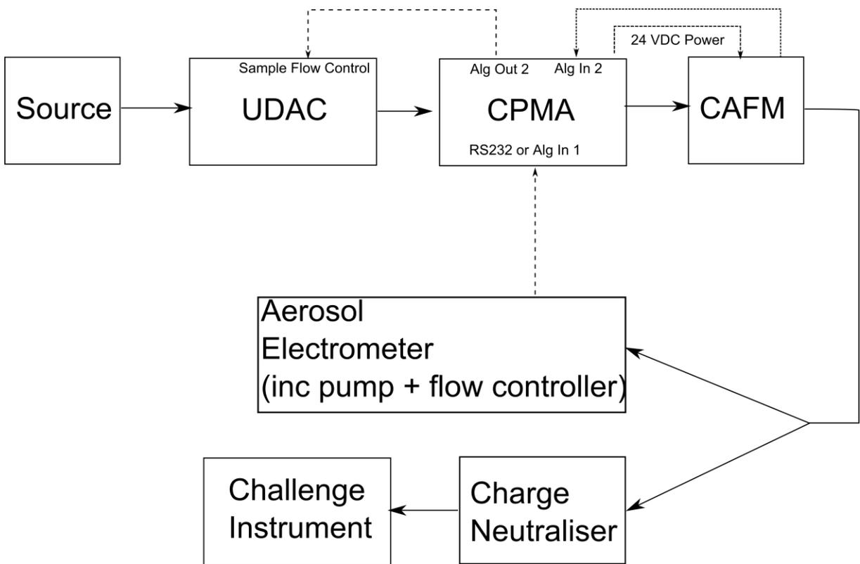
Set the output function of the CPMA to give  $\text{mg}/\text{m}^3$  from the electrometer. This can then be read off the CPMA display or logged to an Output Function File.
