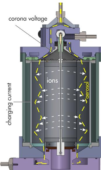
The charger is placed inline as for other aerosol chargers, and the sample flow used in the experiment is either entered on the touchscreen, or measured by the optional Aerosol Flowmeter accessory (see below). The user can specify a constant ion concentration - time product ( $n_t$ ), the charger will calculate and supply the optimum charging current for the given sample flow, temperature and pressure.
