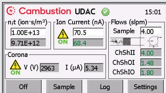
Remote control is possible via text commands to the serial port (or USB via the supplied adapter) or via Ethernet. A built-in webserver provides a Java or VNC based replication of the touchscreen interface to a computer or mobile device.
