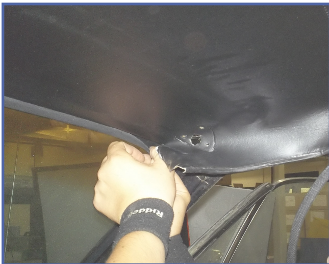
1. Pull material away from Front & Rear windshield windlace
