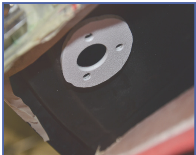
2. Match your holes on your spacer to your original visor mount holes so they align correctly, use double sided tape and stick them on the top of your ceiling between headliner.
