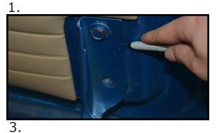
Step 1: Remove your trunk lid and trace hinges so trunk fits exact after install
