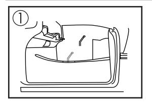
**Step 1:** You will first have to remove your shifter. This is so that we can lay the console over the shifter location.
