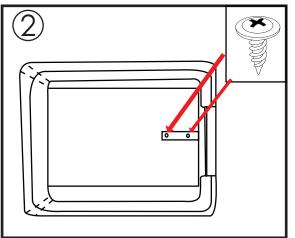
Step 2: Once your TMI Products center console is located in it final position you will lift and remove the bucket in the center console storage compartment. There you will see a tab Resting on the transmission tunnel/floor pan. You will drill two metal screws through the holes in that tab into the trans tunnel/floor pan. Please make sure you have clearance on the other of the tunnel/pan for the screws.
