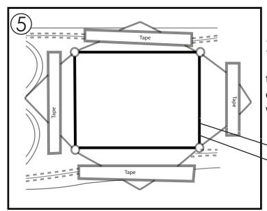
**Step 5:** Once you have pulled back the vinyl you will need to cut the fiber glass. The best way to do this is to use a cut off wheel to cut at all four corners where your guide holes should be drilled you will cut from each guide hole to the other.
