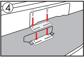
**STEP 4:** Use provided screws to screw in door panel bracket.
