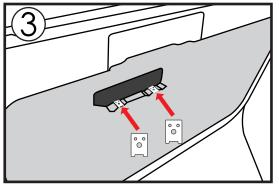
**STEP 3:** Install snap clips to existing door cup holes.
