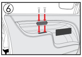
**STEP 6:** Install door cup kit using supplied screws. Install complete.
