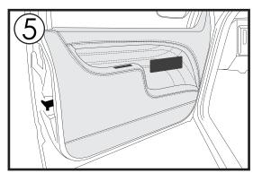
**STEP 5:** Fit door panel using supplied clips with lower factory holes.
