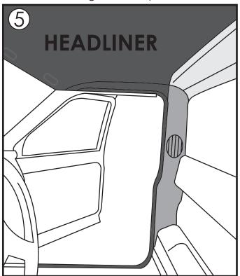
**STEP 5:** Install TMI Headliner. Note: You may need assistance holding the Headliner as you reinstall factory trim and A pillars.
