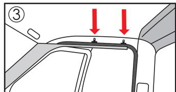
**STEP 3:** Use pry tool to remove A pillar making sure not to break the clips under the A pillar. Use the pry tool in a twisting motion. Prying on the pillar could cause it to break.
