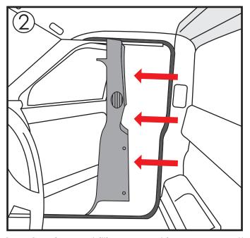
**STEP 2:** Using a Phillips screwdriver, remove the screws attaching the rear speaker trim.
