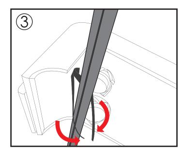
STEP 3: Use the Velcro strap to wrap around the rear bar multiple times to prevent movement of the center console.
