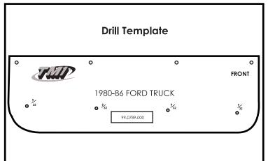
**Step 2.** Cut out the provided template following the scissors as well as all the labled holes/openings.
