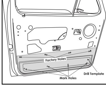
**Step 3.** Align the template to the factory holes.
