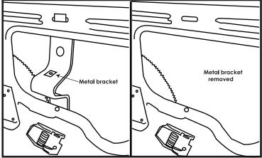
**Step 7.** Remove the metal door mount bracket.
