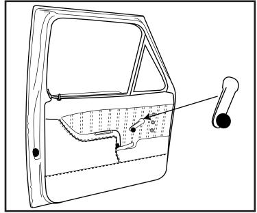
**Step 11.** Mount the window crank handle.
