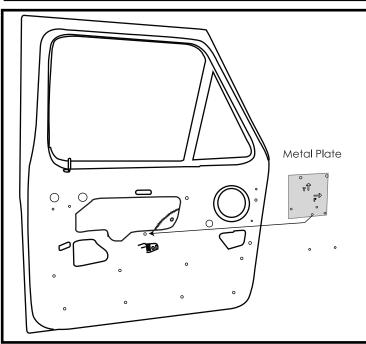
**Step 8.** Use the hole that held the metal bracket to line up the metal plates bottom screw hole. Mount the metal plate with the provided screws.
