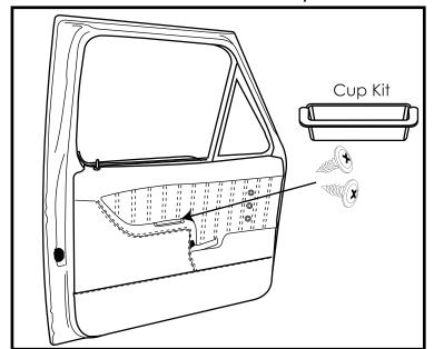
**Step 10.** Slide the door panel into the window track. Snap the bottom clips into the 9/32 in drilled holes. Use the 2 provided screws and mount the cup kit.
