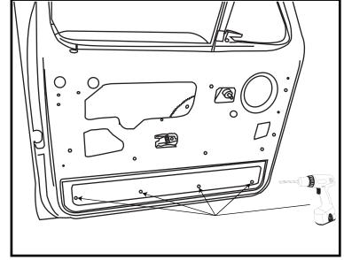
**Step 6.** Drill out the marked holes using the sizes indicated on the drill template.
