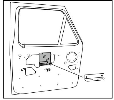
**Step 9.** Mount the door panel cup kit bracket to the metal plate using the screws provided. **NOTE: Bending the bracket to properly fit the**
