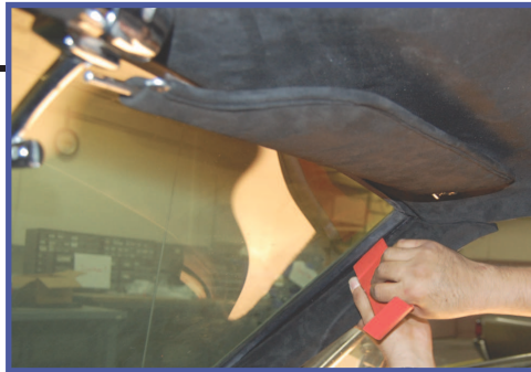
Using the Plastic Trim Tool, tuck the A-Pillar cover into the windshield window seal.
