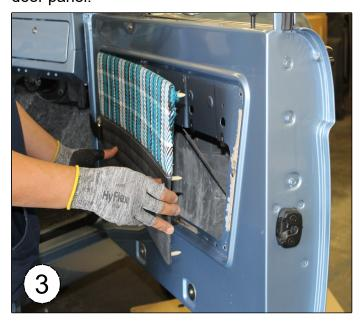
2. Your new TMI panel will have the factory holes pre-cut to install factory hardware. If arm rest and door handle cup will not be used, do not cut the upholstery material.
