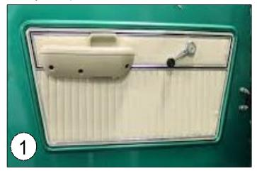
3. Install new panel using the provided drill templete to mark and drill out the holes to acomadate the christmas tree style clips on new door panel.
