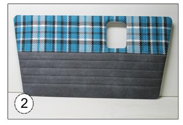
Once panel is in place, cut a slit for the cranks.
