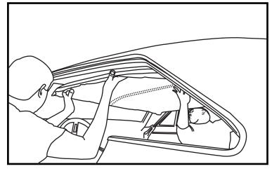
Step 3. Starting from the drivers side, slide the headliner into the vehicle. Make sure the headliner is over the top of the dash board and steering wheel.
