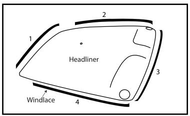
**Step 7.** Install the original windlace (pinch molding) starting with number 1 and ending with number 4.
