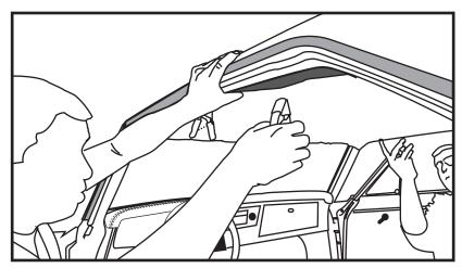
Step 6. Using 4 spring clamps, clamp the headliner to the roof of the vehicle. Put 1 clamp in the front top of the door opening for the driver side and 1 clamp for the passenger side. Put 1 spring clamp towards the back top of the door opening for the driver side and 1 clamp for the passenger side.
