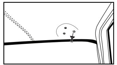
**Step 9.** Using a needle or tack locate the 3 screw holes to mount the left and right visors.
