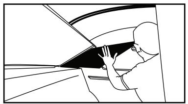
**Step 8.** Snap in the sail panels on the left and right rear of the vehicle.
